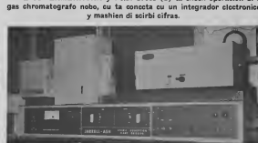
THE LAB'S newest piece of equipment is this atomic absorption spectrophotometer. It will determine lead, sodium, and vanadium in hydrocarbons rapidly and precisely.
